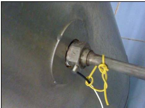
Figure 2: Position of SENSOR1 on the temperature gauge. Note the yellow rubber band for additional fixing of the sensor. Photo by D. Varner
