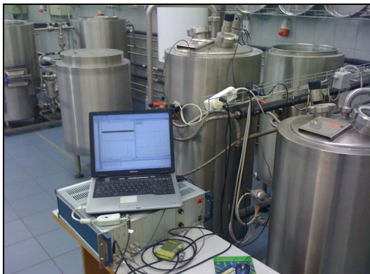
Figure 5: Control laptop PC on top of XEDO AE analyzer. Photo by D. Varner
