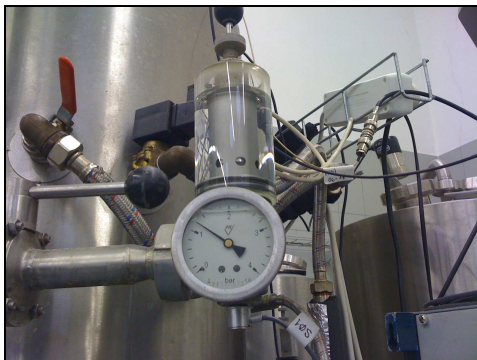
Figure 3: Position of SENSOR2 on the carbon dioxide outlet valve assembly. The sensor can be seen below the gauge dial, glued upside-down to the bottom of the assembly. Photo by D. Varner
