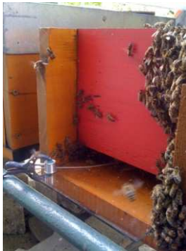
Figure 3: Slot02 sensor on the glass plate in the inlet port. Photo by authors.
