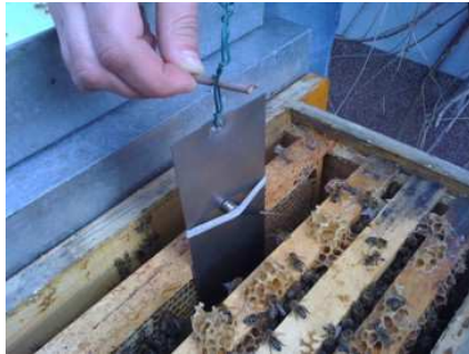
Figure 2: Slot01 sensor on the sheet metal plate in the hive interior. Photo by authors.
