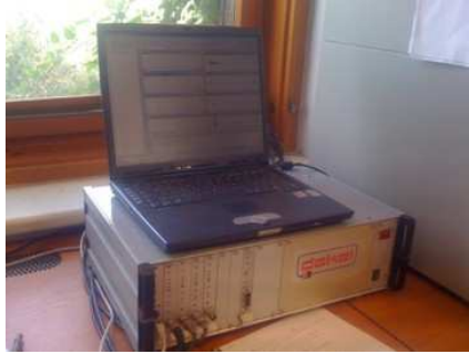
Figure 4: Dakel XEDO AE analyzer used in the experiment. Photo by authors.
