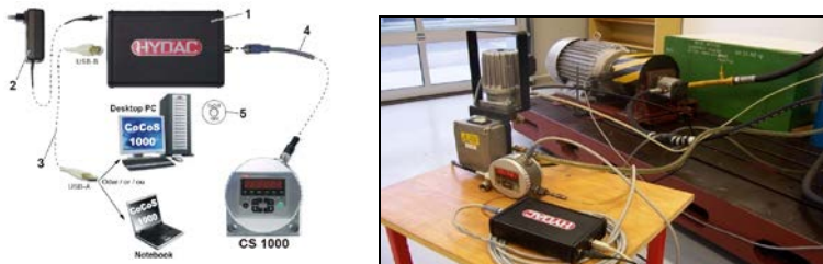
Fig. 2 Wiring diagram of CS 1000 device 1-Adapter, 2-Modul of power box, 3-USB cable, 4-CS 1000 and connecting cable, 5-software pack CoCos 1000
