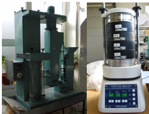
Fig. 1 Laboratory screening machine K-293 with vertical air flow (left) and Haver EML digital plus Test Sieve Shaker (right)
