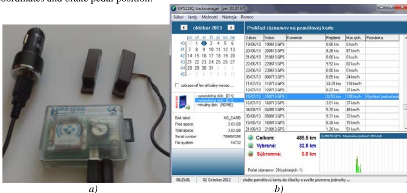
Fig. 2 Device detecting an effect of driver on fuel consumption: a) connection of individual parts, b) software for loggings assessment
