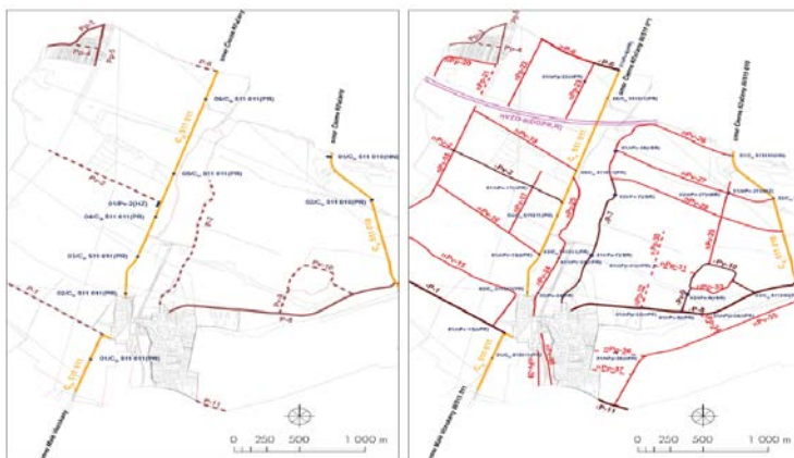
Fig. 2: Reconaissance of existing field road in project perimeter (left), new design of transportation facilities and measures in the project's perimeter (right)
