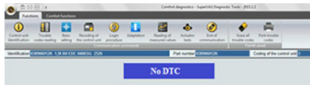
Figure 7 Diagnostic Trouble Codes of the ECU – No DTCs
