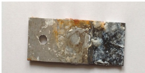
Figure 2 Corrosive specimen after being subjected to corrosion process in salt-spray chamber
