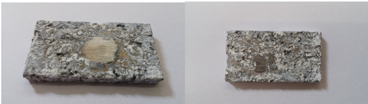
Figure 5 The sample after 144 hours of accelerated corrosion degradation (refined)
