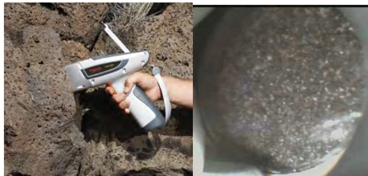
Figure 1 Analyser Thermo Scintigic Nitron XL3 Gold
