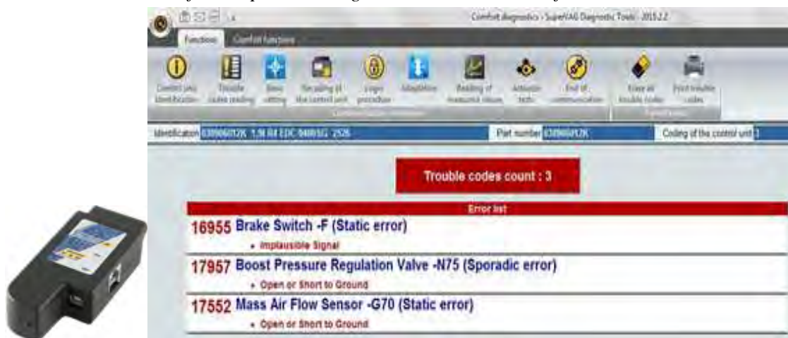
Figure 3 Demonstration of the SuperVAG diagnostic hardware and software
