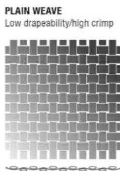
Figure 1 The most common version of bidirectional weave (plain weave)
