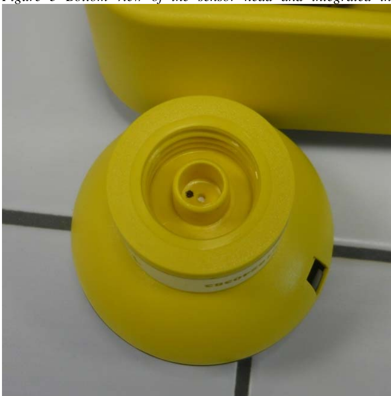
Figure 3 Bottom view of the sensor head and integrated in the pressure-sensitive membrane
