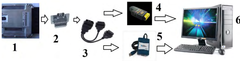
Figure 6 Data mining scheme ECU BOSCH EDC17CP20
