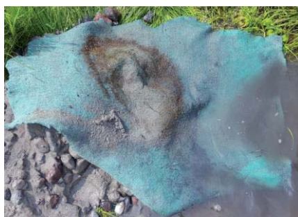
Figure 2 The tested nonwoven geotextile after exploitation in the Białobrzegi earthfill dam
