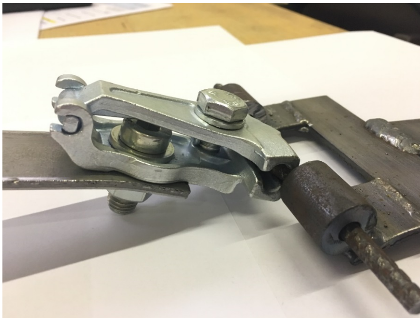
Figure 6 Deformation of the tested clamp
