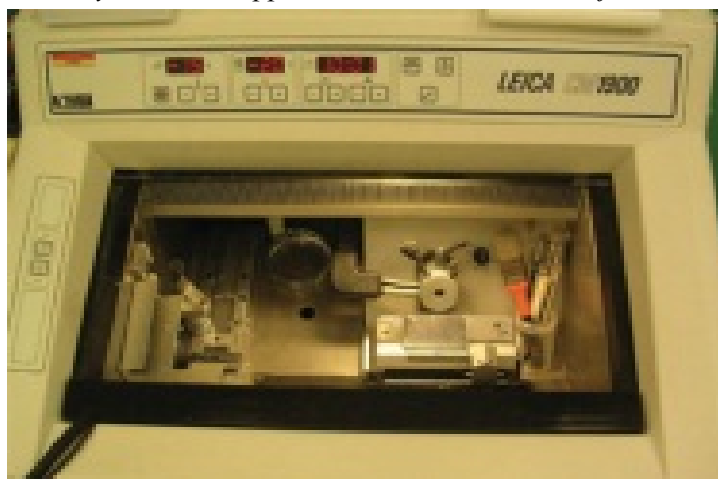
Figure 1 The Leica CM1900 Cryostat –this apparatus was used to section frozen tissue onto slides
