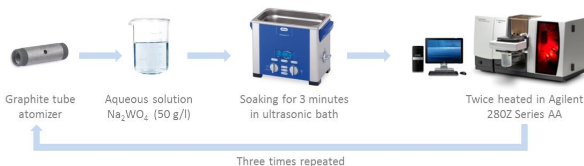
Figure 1 Scheme of graphite furnace surface-modification
