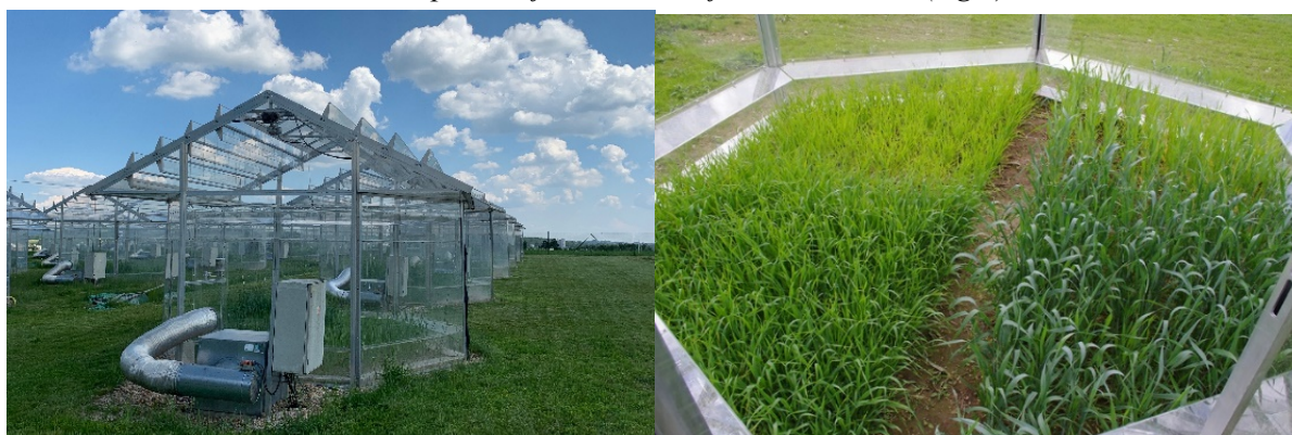
Figure 1 Open top chambers for manipulation of CO 2 concentration and water availability (left) and view inside the chamber with plots unfertilized and fertilized with N (right).
