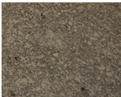
Figure 2 Hardened C45 steel structure
