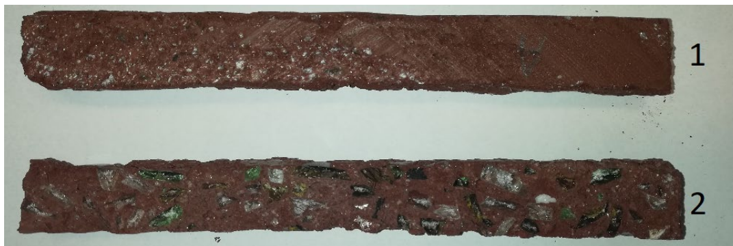
Legend: 1 – Sample with the admixture of glass with larger grain size, 2 – sample with admixture glass with a smaller grain size
